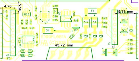
Refer to drawing above for the maximum dimensions of the internal PCB and pin spacings. The terminal strip spacings are standard 2.54mm/0.1". The carrier board contains receptable headers so the expansion board needs to have pin headers.
